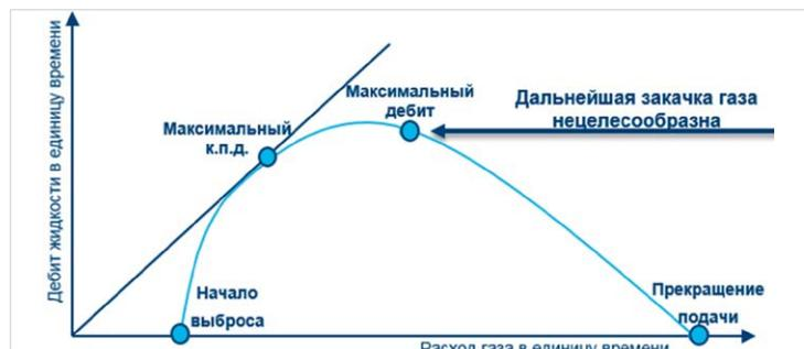
Fig. 3 — The relationship between the flow rate of the liquid and the gas flow
